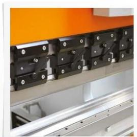
**Promecam Top Tool Clamping System (S)**
